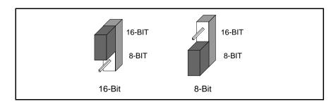
Figure 2-11. Jumper Settings for 8-Bit and 16-Bit Mode Operation
